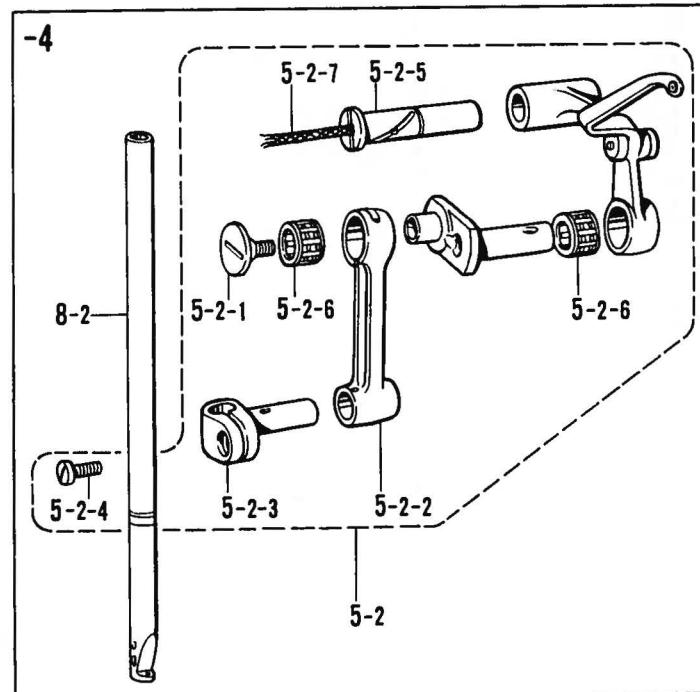
B. 針棒関係 /Needle bar mechanism/Nadelstangenvorrichtung/
