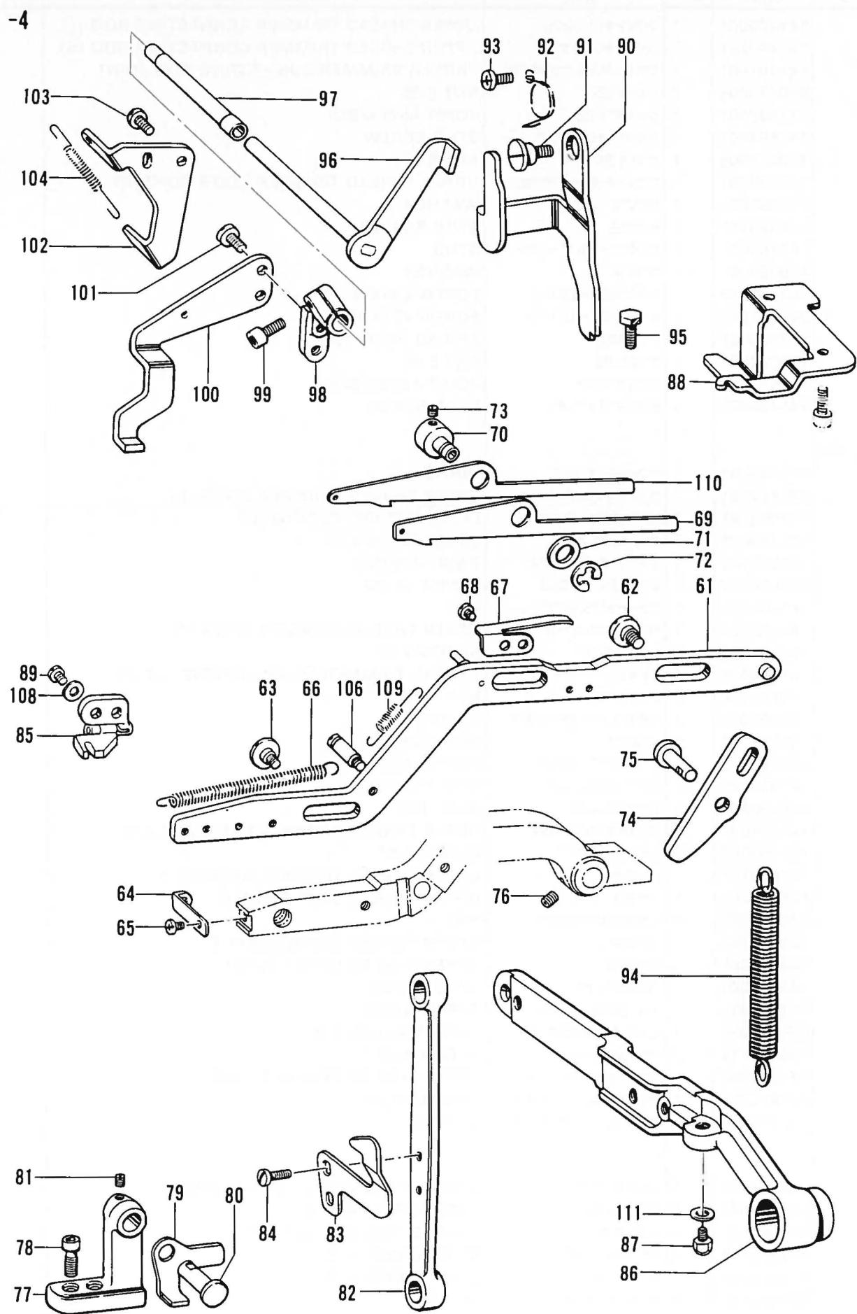
W. 上糸切り関係 (2) /Upper thread trimmer mechanism (2)/Oberer Fadenabschneider (2)/
