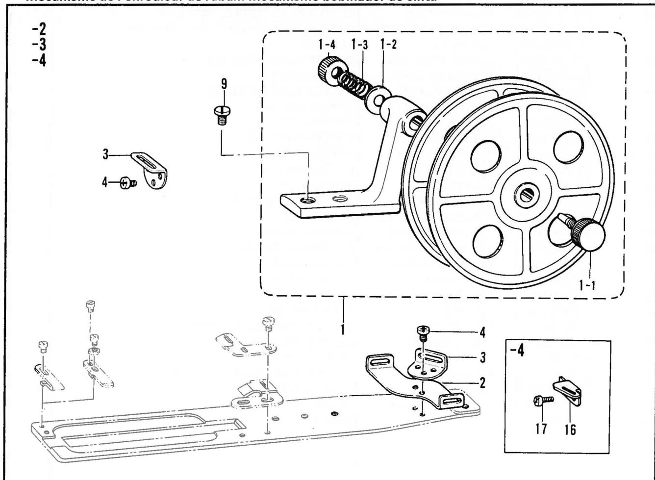
P. 糸切レ感知関係 / Thread breakage detector mechanism / Fadenbruchfühler /
